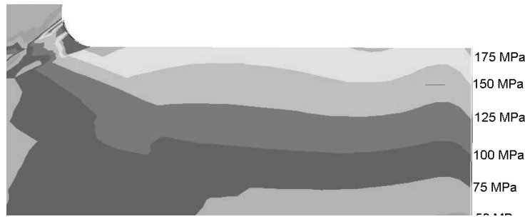
Figure 5 - Stresses calculated by Finite Element in the legs of the Standard Reference
